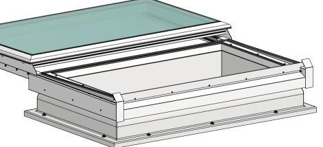
L = OPENING LENGTH (MAX 250 cm FOR SMOKE VENTILATION) W = OPENING WIDTH (MAX 130 cm FOR SMOKE VENTILATION) H = UPSTAND HEIGHT (MIN 25 cm FOR SMOKE VENTILATION) a = ABOUT 2 cm SLOPE FOR WATER OUTFLOW
